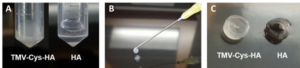
Figure 1.7. Illustration of the in situ hydrogel formation. (A) The pre-hydrogel mixture with TMV1cys (left) and without TMV1cys (right). (B) Injectable simulation of pre-hydrogel mixture through needle 20G. (C) The TMV1cys-based HA hydrogel (left) and HA hydrogel (right) after gelation for 2 h.
